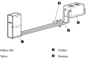
Note: Install isolation valves and particulate strainers with 20 mesh stainless steel screen (opening size = 865 micron) in the supply line between the chiller and RC.
